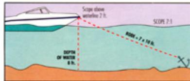
Make sure the bitter end of the anchor line is attached to boat before dropping the anchor. Bring the bow into the wind
