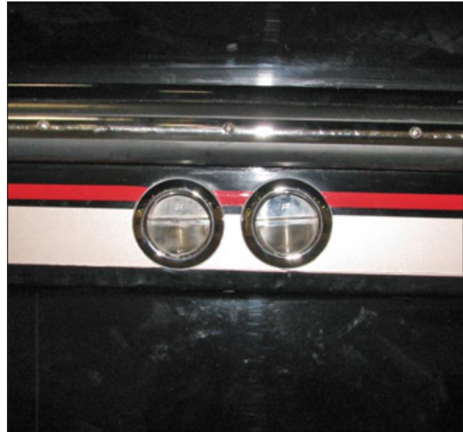
Scupper Drain Thru-Hull Fittings & Check Valves
