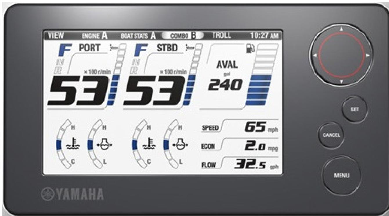
Yamaha Command Link Plus® / Typical Two Engine Combo Screen For Quad Engines
