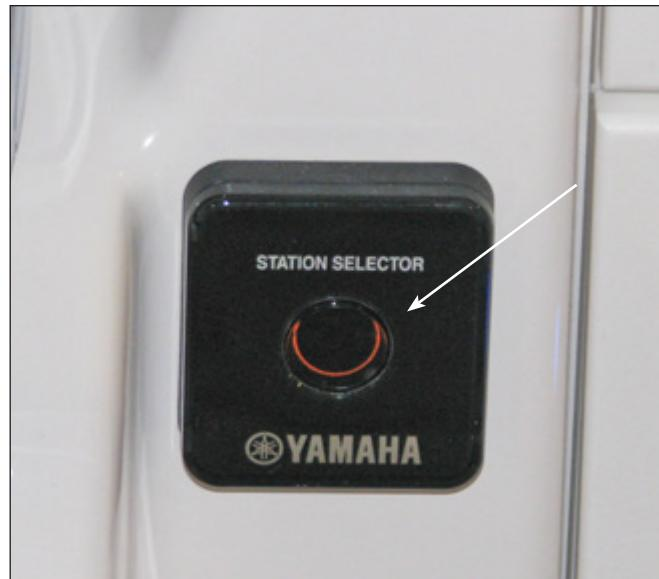
Typical Yamaha Triple Engine Station Transfer Button
