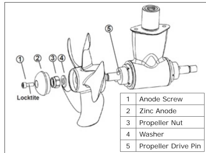
Bow Thruster Anode & Propeller Assembly
