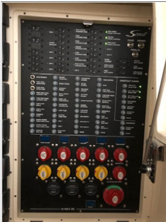
Quint Engine Battery Switch Panel, Motorized Battery Switches, Remote Battery Switches, Parallel Switches & Circuit Breakers
