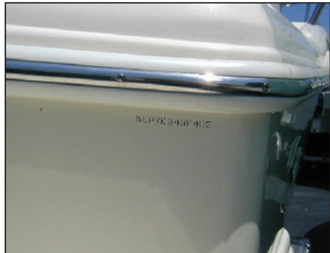
Typical Hull ID Number on Starboard Transom
