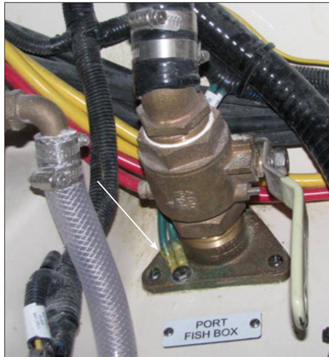
Thru-Hull Valve Bonding Wires & Connection
