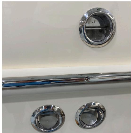
Scupper Drain Thru-Hulls
