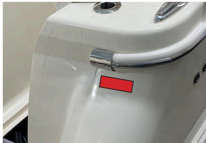
Typical Hull ID # Location on Starboard Transom
