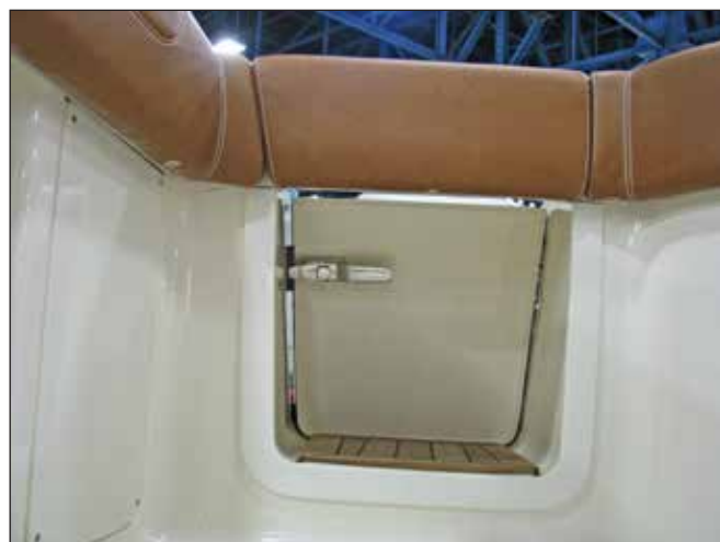
Transom Door Latch & Push Button Safety Pin
