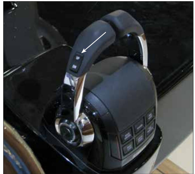
Yamaha Quad Engine Port Control Trim Switch
