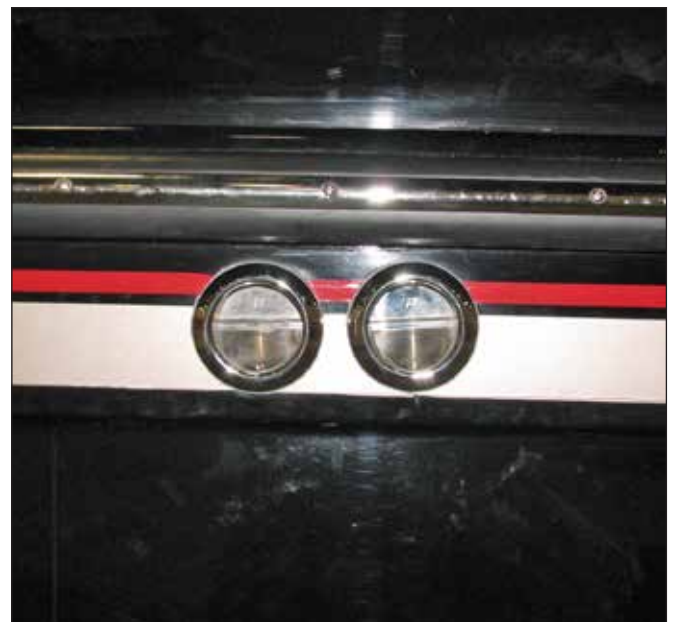
Scupper Drain Thru-Hull Fittings & Check Valves
