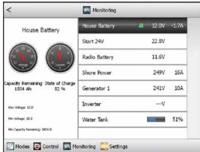
CZone Display Monitoring Screen
