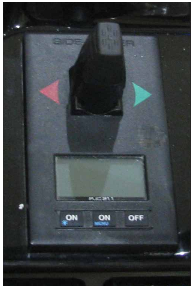
Typical Bow Thruster Control Panel
