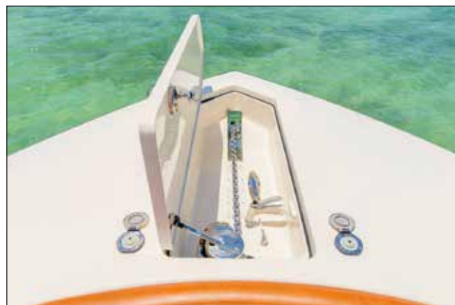
Windlass Compartment Washdown Hose
