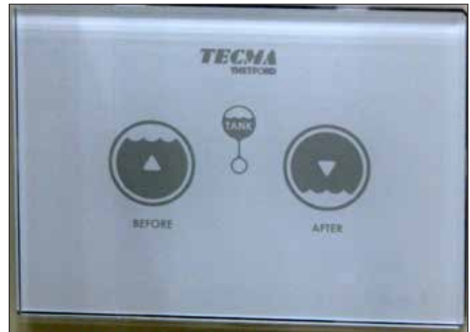
Typical Marine Head Control Panel & Tank Monitor
