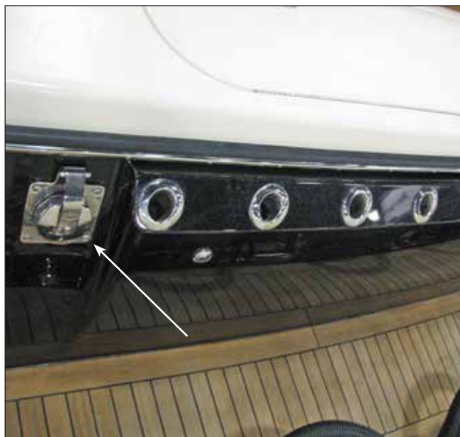
Shore Power Inlet Cord Hawse Pipe
