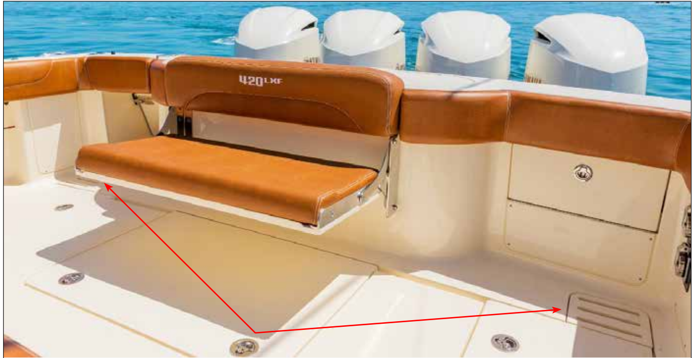
Port & Starboard Cockpit Scupper Drains
