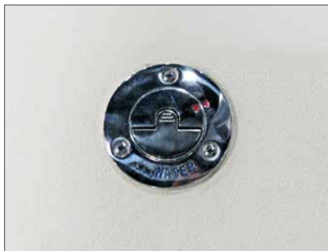
Fresh Water Tank Deck Fill Plate
