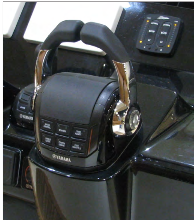
Typical Yamaha Quad Engine Electronic Controls
