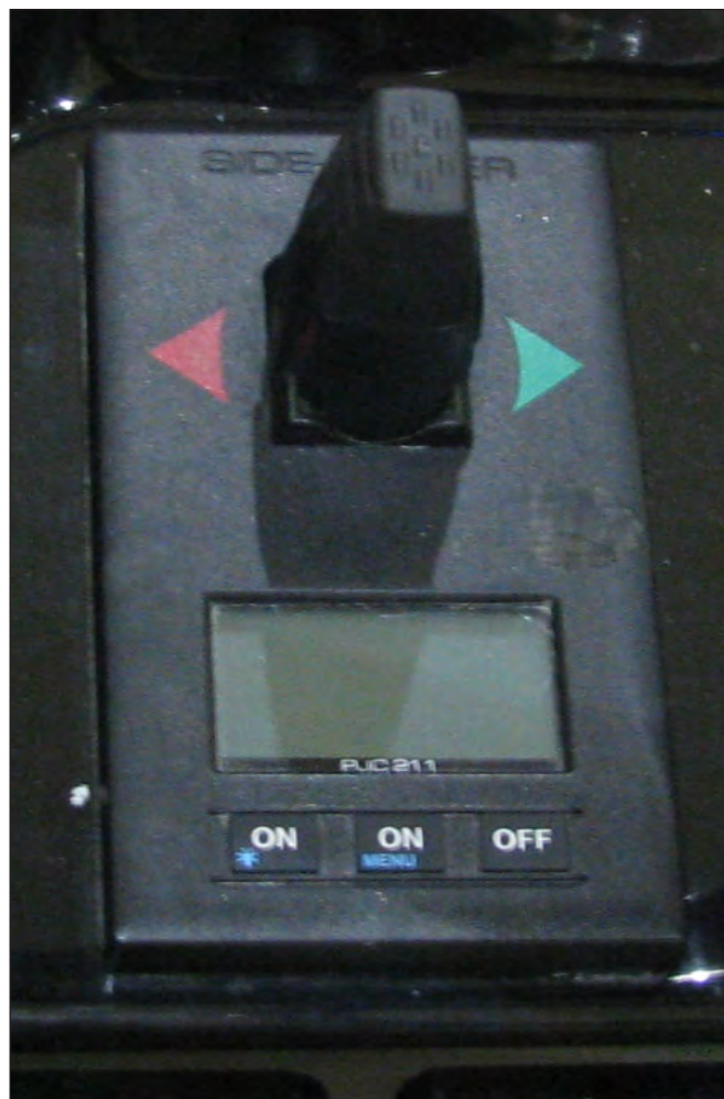
Typical Bow Thruster Control Panel
