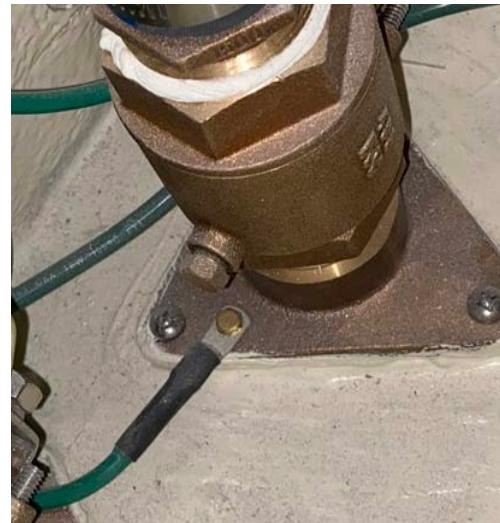
Thru-Hull Valve Bonding Wires & Connection
