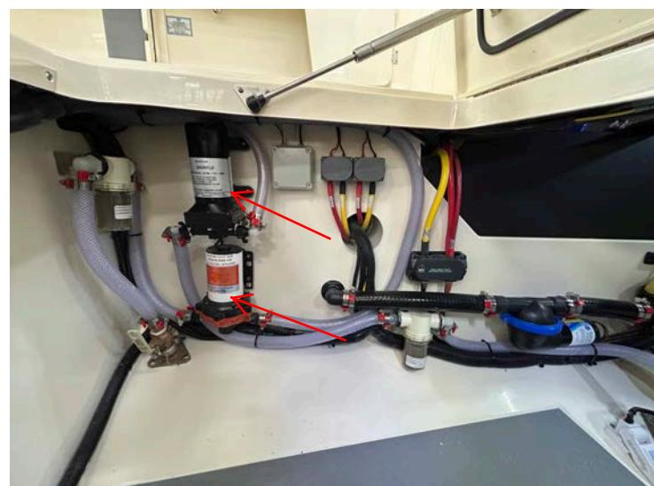
A/C Cooling and SeaKeeper Pumps
