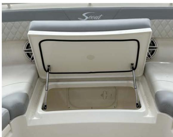
Center Bow Storage Compartment & Anchor Locker Access Hatch
