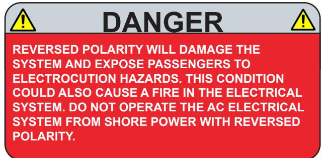
If the reversed polarity light is lit or the ELCI continues to trip and the red "FAULT" LED is lit after being reset there is a problem with the AC electrical system and it is unsafe to use. Make sure all AC accessory circuits are OFF and turn the Shore Power main breakers OFF. Then turn the shore power inlet panel main and the dockside circuit breakers OFF.
