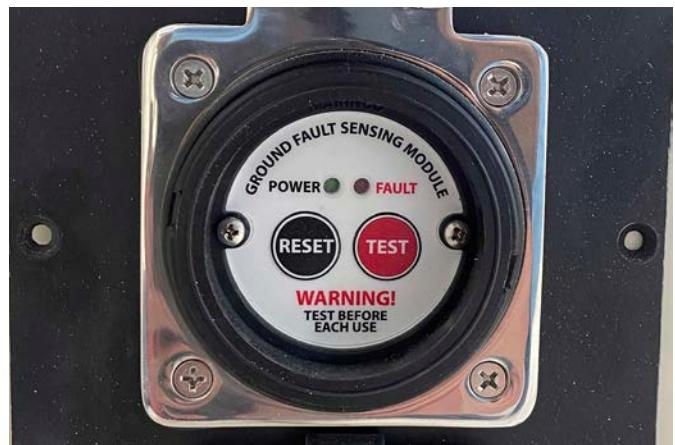
ELCI Inlet Panel & TEST/RESET Buttons
