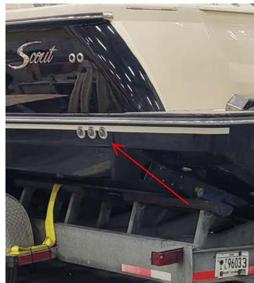
Scupper Drain Thru-Hulls
