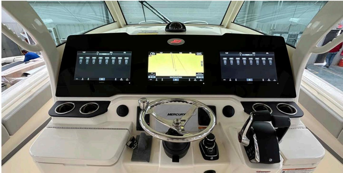
Switch Panel In Helm Electronics Touch Screen Display Panel
