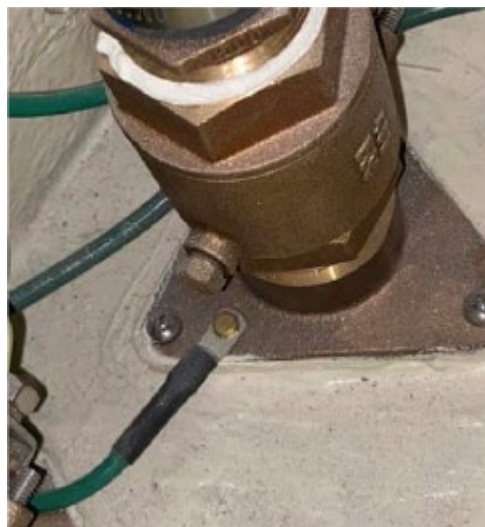
Thru-Hull Valve Bonding Wires & Connection
