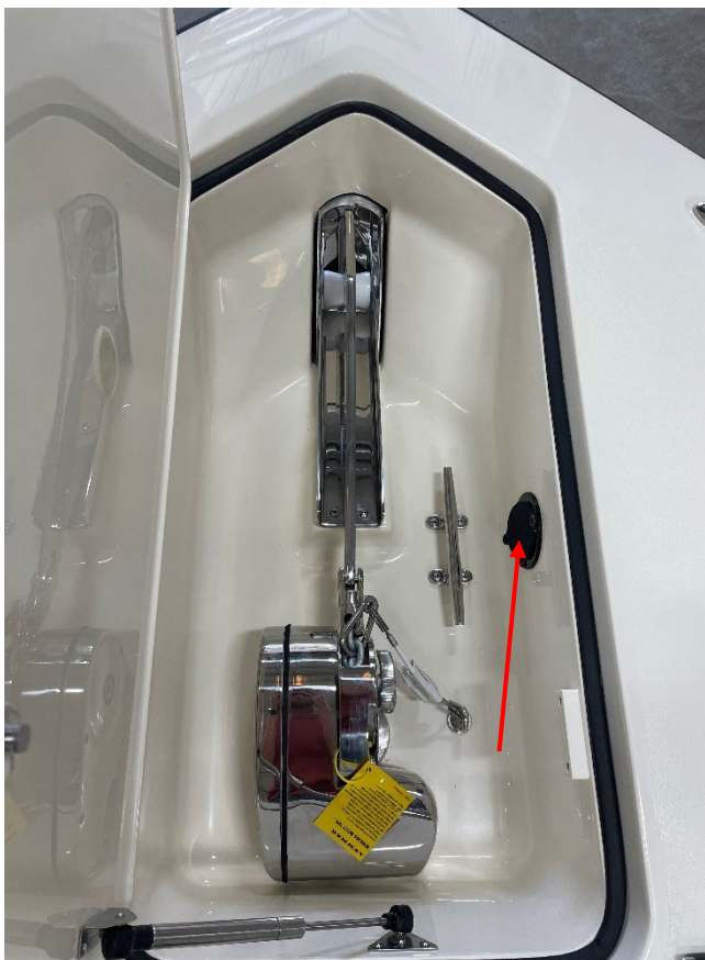
Windlass Compartment Washdown Quick Disconnect
