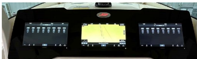
Switch Panel in Helm Electronics Touch Screen Display Panel
