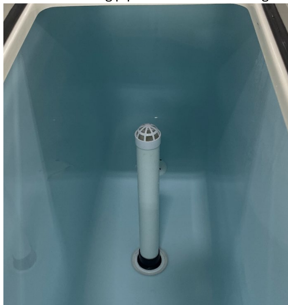
Baitwell with standing pipe installed
