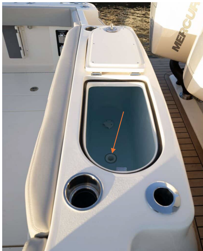
Transom Baitwell and drain fitting
