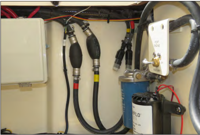
Triple Engine Fuel System - Port Engine Fuel Filter, Fuel Selector Valve & Primer Bulbs
