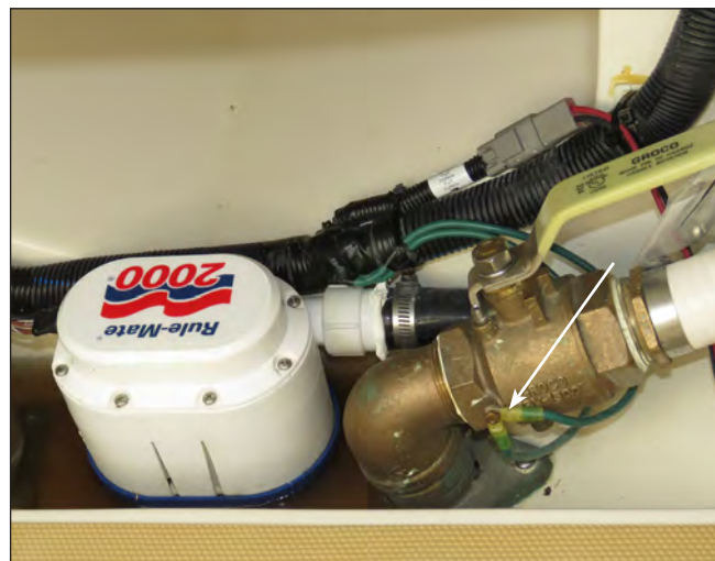
Typical Bonding Wire Connection
