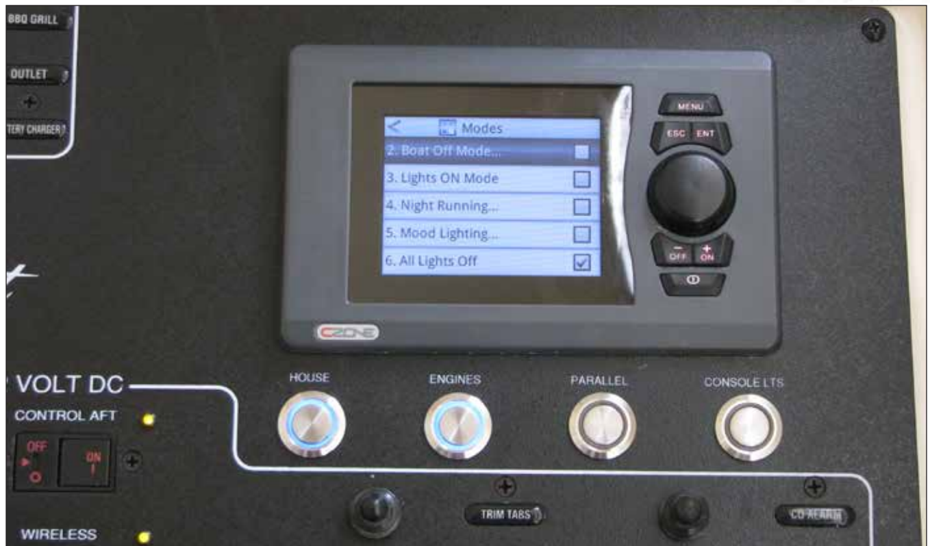
Battery & Parallel Remote Switches - House & Engine Battery Switches On CZone Control Panel
