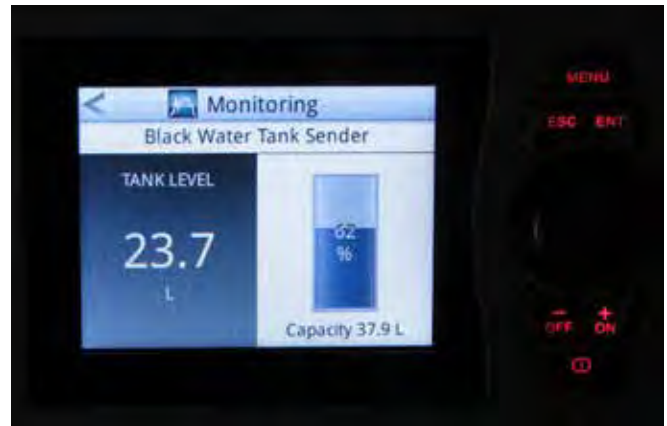
CZone Holding Tank (Black Water Tank) Fluid Level Monitor
