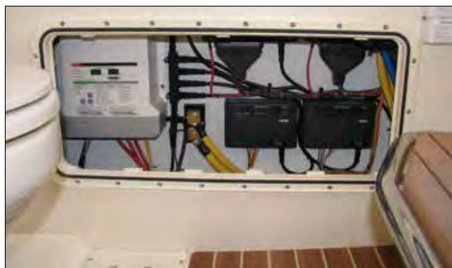
Forward Bilge Compartment, Battery Charger & Control Modules
