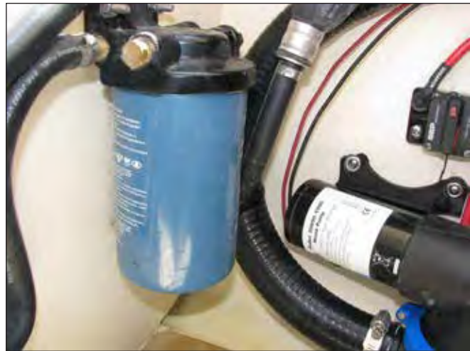
Engine Fuel Filter In Aft Systems Station
