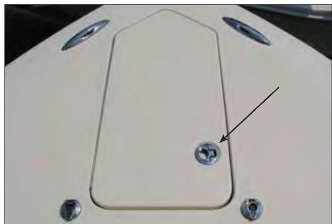
Anchor Locker Hatch Twist Lock Latch Handle can be stored flush to hatch only when latched
