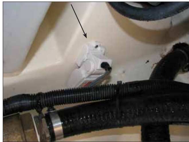
High Water Alarm Automatic Float Switch
