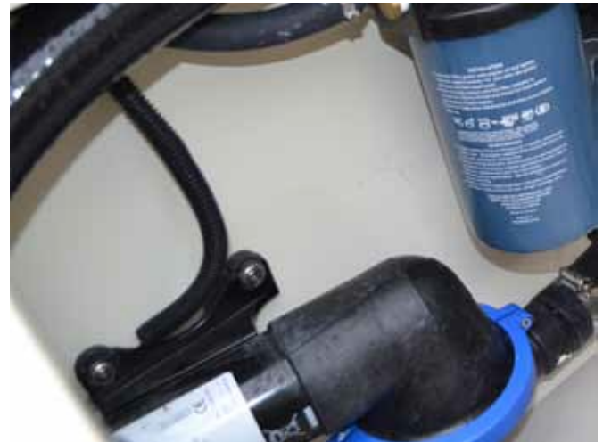
Overboard Discharge Pump in Stern Bilge
