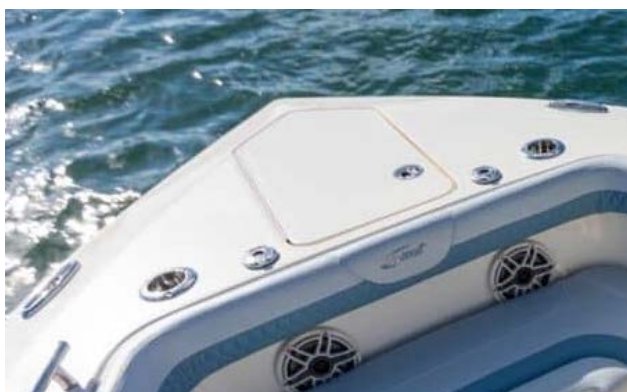
Windlass IN & OUT Switches
