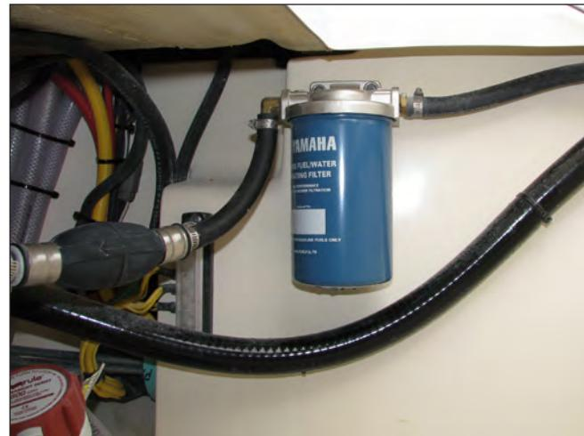
Engine Fuel Filter & Primer Bulb In Aft Systems Station
