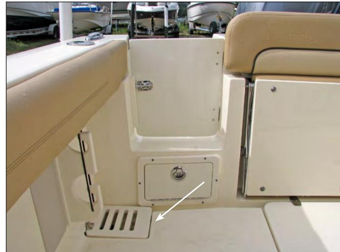
Starboard Cockpit Scupper Drain
