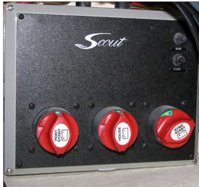
Twin Engine Battery Switch Panel
