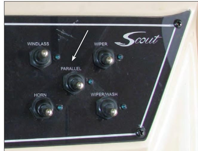
Parallel Switch In Helm Switch Panel
