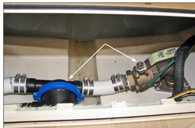
Waste Discharge Pump & Thru-Hull Valve
