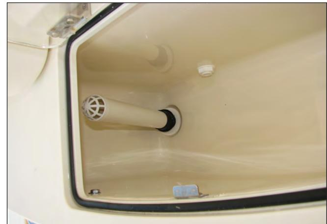
Leaning Post Baitwell Standpipe & Drain Fitting
