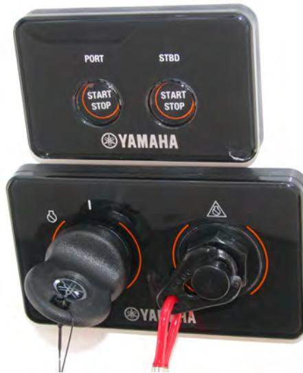
Typical Twin Engine Yamaha Command Link Plus Ignition & Start/Stop Switch System
