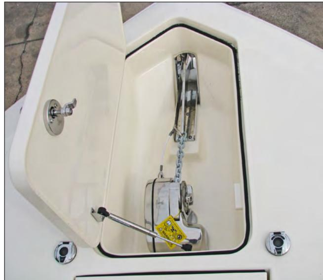
Windlass, Deck Foot Switches, Bow Roller & Chain Binder
