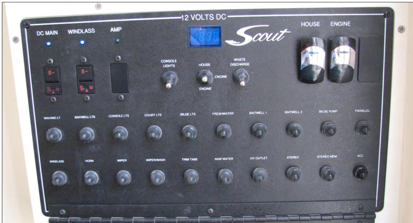
DC Breaker Panel & Remote Battery Switches
