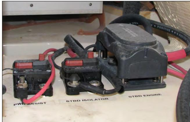
Typical Yamaha Engine Charging Circuit & Power Assist Steering Heavy Duty Circuit Breakers
