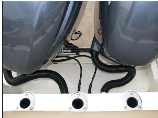
Typical Twin Engine Steering Cylinders & Tie Bar
