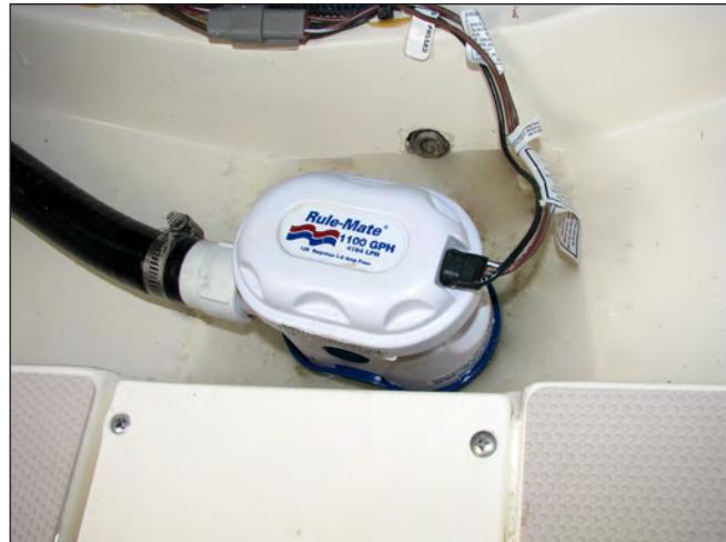
Bilge Pump W/ Built In Automatic Switch
