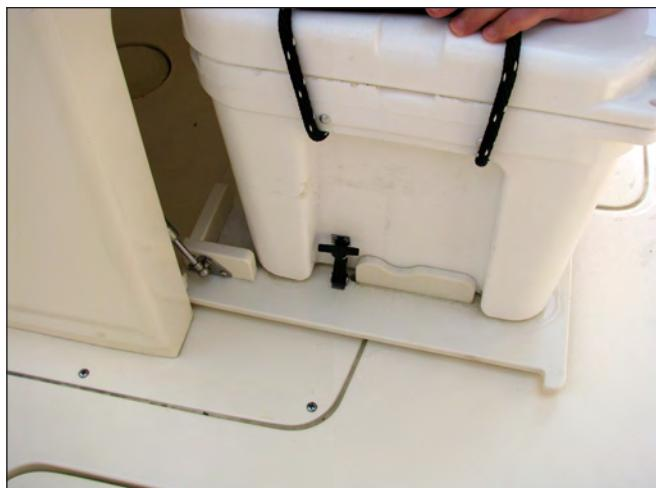
Cooler Slide Assembly & Draw Latch
