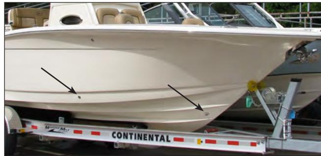
Forward Fishbox/Storage Compartment & Rope Locker Drains
