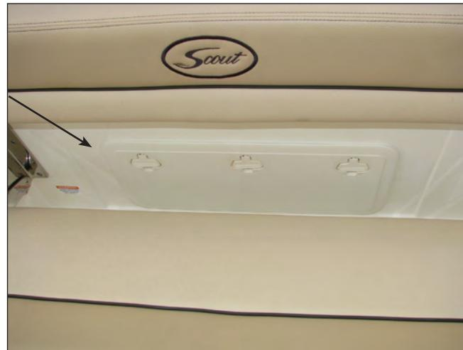
Aft Electrical Systems Compartment Hatch
