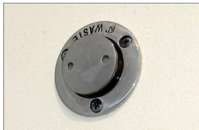
Waste Deck Fitting - Cap Released & Providing Handhold
