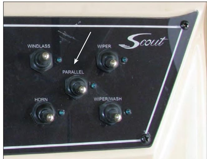
Parallel Switch In Helm Switch Panel
