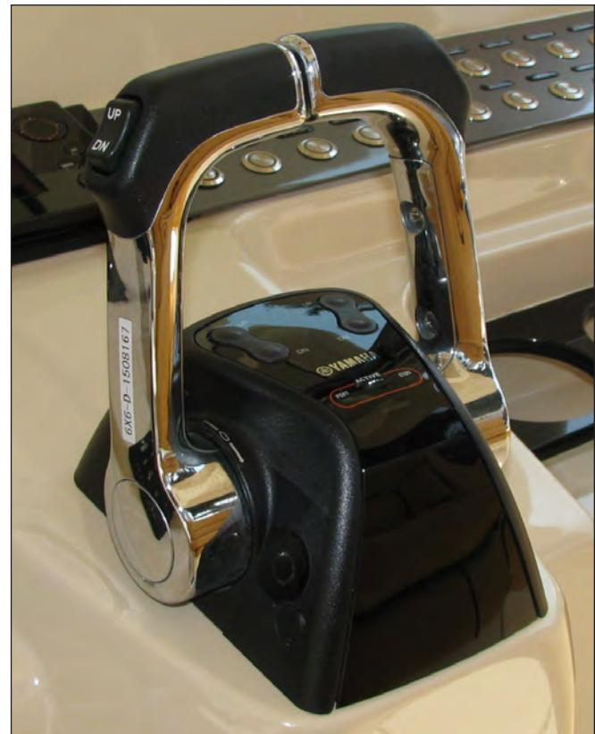
Typical Yamaha Twin Engine Electronic Controls
