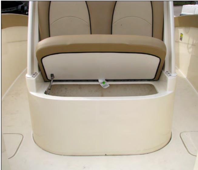
Forward Console Seat Cooler Hatch
