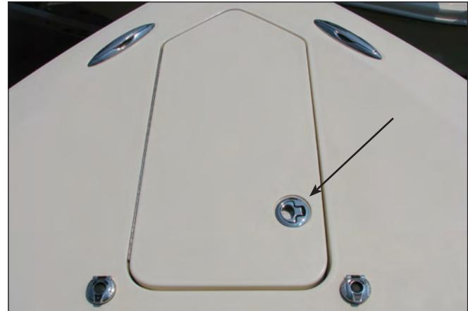
Anchor Locker Hatch Twist Lock Latch
