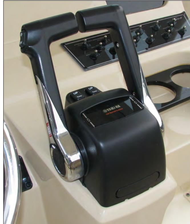
Typical Twin Engine Cable Controls
