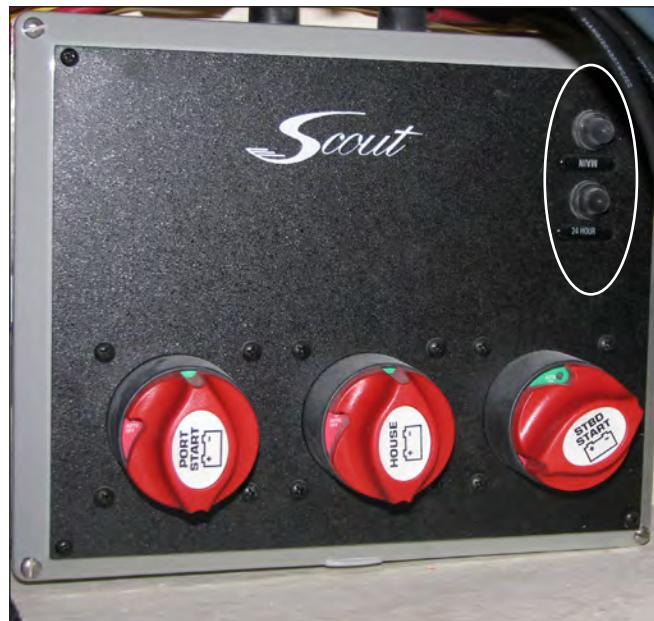
Twin Engine Battery Switch Circuit Breakers
