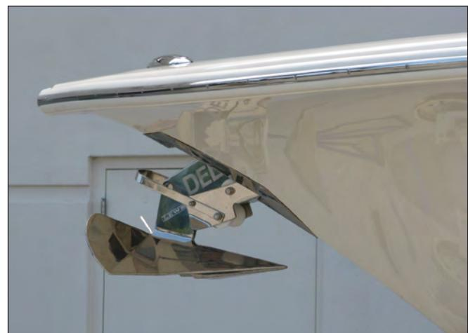
Anchor Roller & Delta Plow Anchor
