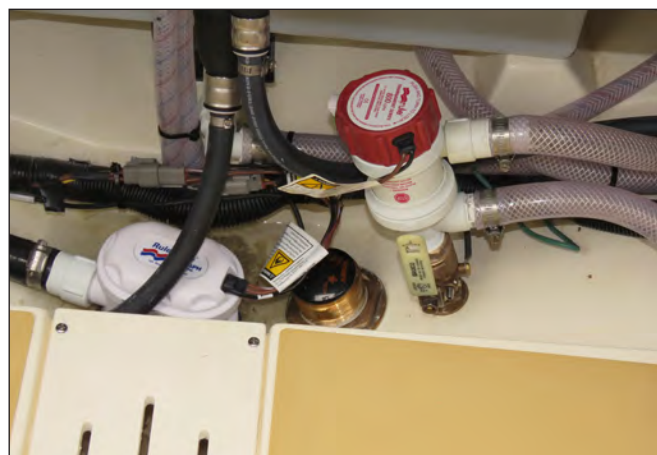
Baitwell Pump, Seacock Valve & Auxiliary Supply Fitting
