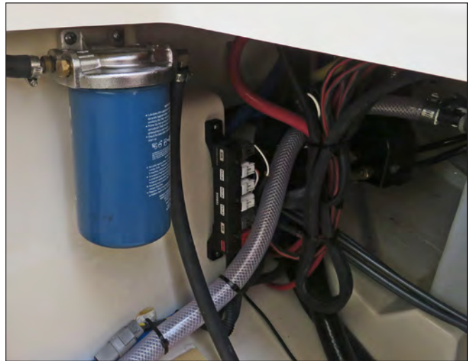
Engine Fuel Filter In Aft Systems Compartment
