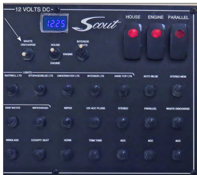
Waste Discharge Switch In DC Breaker Panel
