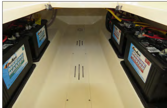
Typical Twin Engine Starting & House Batteries In Ski/ Battery Storage Compartment Below Cockpit Sole
