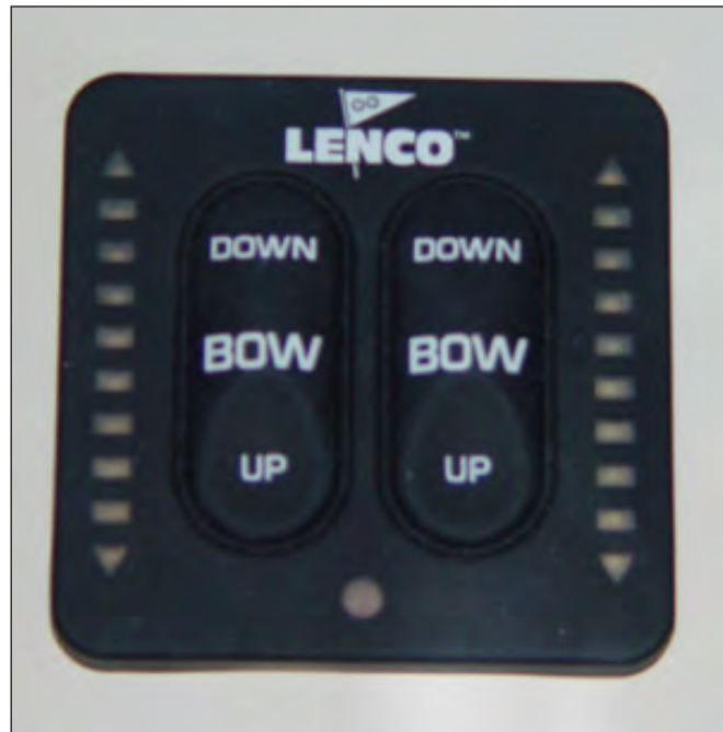
Optional Trim Tab Control Switches & LED Indicators
