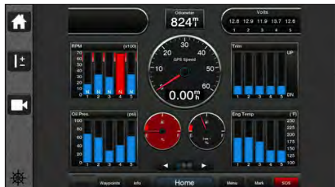
Typical Garmin Display Engine Data
