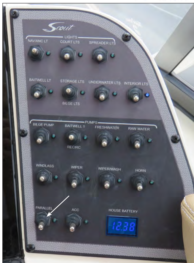
Helm Switch Panel & Parallel Switch
