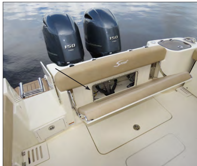
Aft Electrical Systems Compartment Behind Stern Bench Seat
