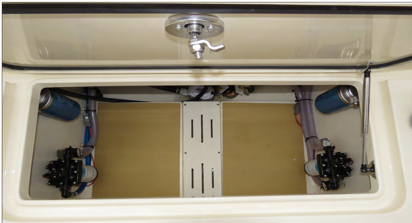
Aft Systems Compartment Showing Hatch Drain Rails & Bilge Pump
