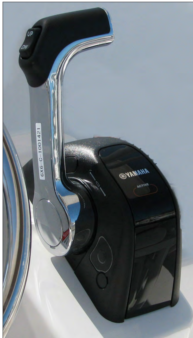
Typical Yamaha Single Engine Electronic Control
