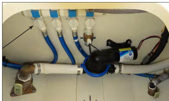
Fresh Water Manifold & Control Valves In Ski/Battery Storage Compartment
