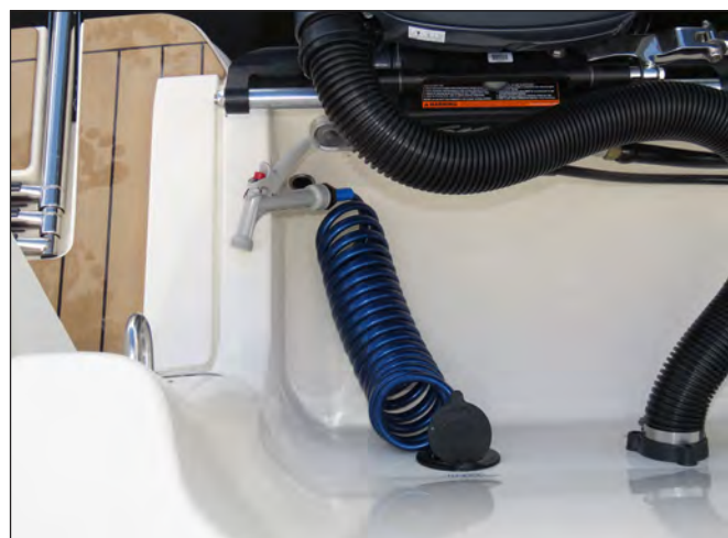
Cockpit Fresh Water Washdown Hose & Connection
