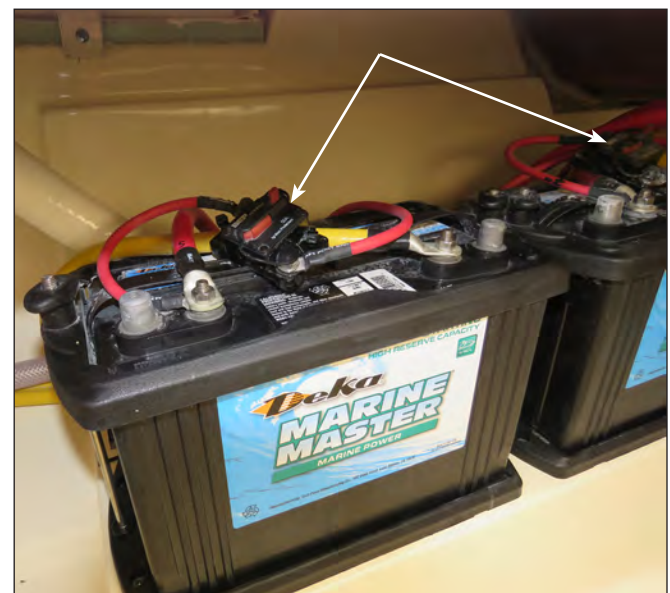
Engine Starting Battery Charging Wire Circuit Breakers
