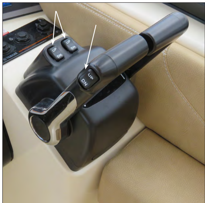
Typical Yamaha Twin Engine Cable Control Trim & Tilt Switches
