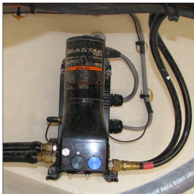
Typical SeaStar Steering Power Assist Pump & Reservoir
