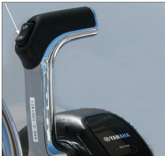
Typical Yamaha Single Engine Trim & Tilt Switch
