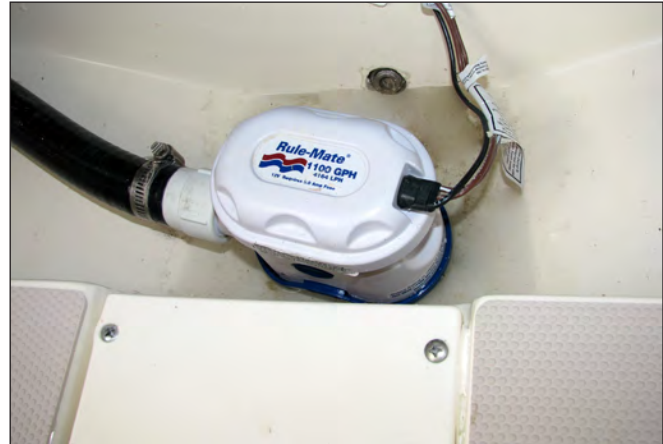
Bilge Pump W/ Built In Automatic Switch In Aft Systems Compartment
