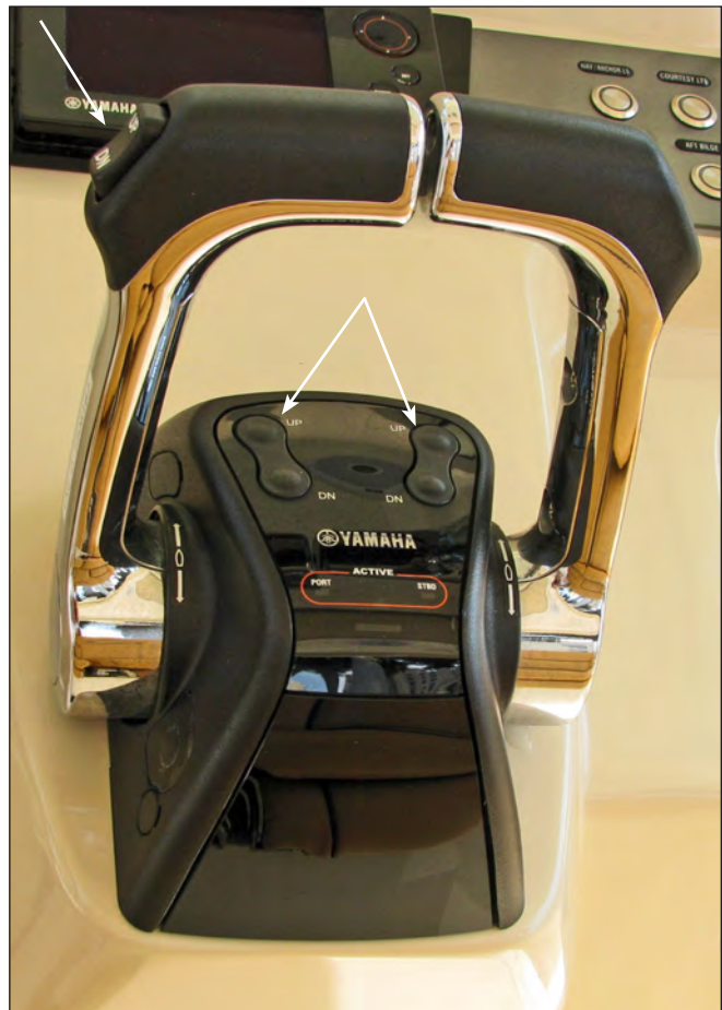
Typical Yamaha Twin Engine Electronic Control Trim & Tilt Switches
