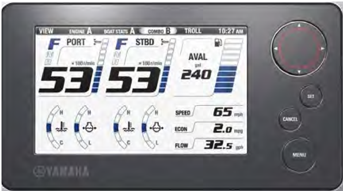
Yamaha Command Link Plus® / Twin Engine Combo Screen
