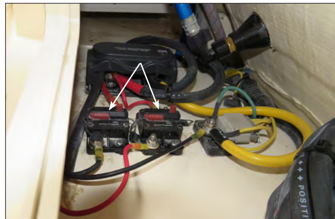
Typical Engine Charging Circuit & Power Steering Pump Circuit Breakers Located Behind The Aft Bench Seat.
