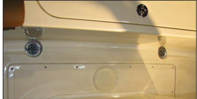
Scupper Drains & Drain Rails
