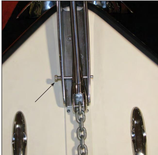
Anchor Safety Pin in Bow Roller Assembly
