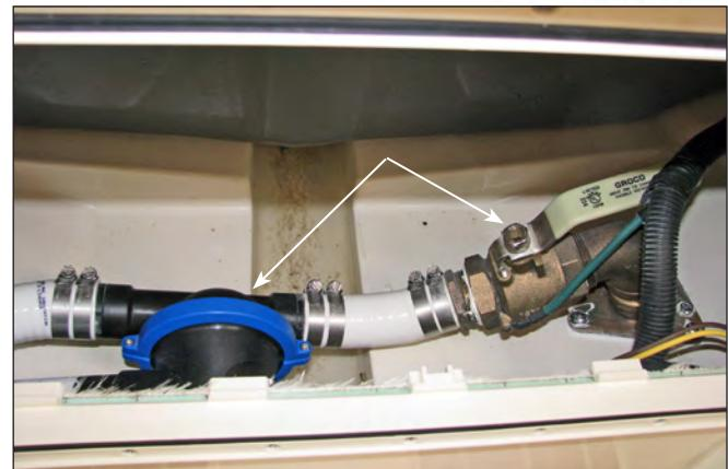
Typical Waste Discharge Pump & Thru-Hull Valve
