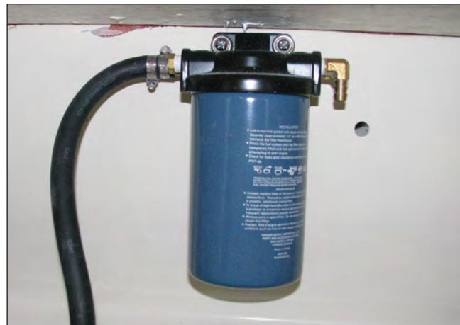
Typical Remote Outboard Engine Fuel Filter
