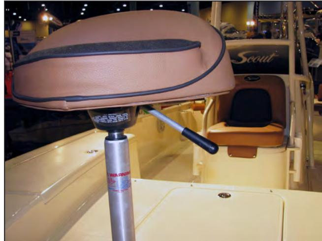
Casting Seat Height Adjustment Lever
