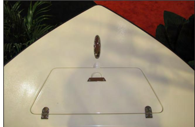
Anchor Locker Deck Hatch & Retractable Cleat
