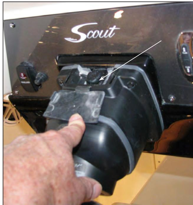
Typical Hydraulic Steering Helm & Filler Cap
