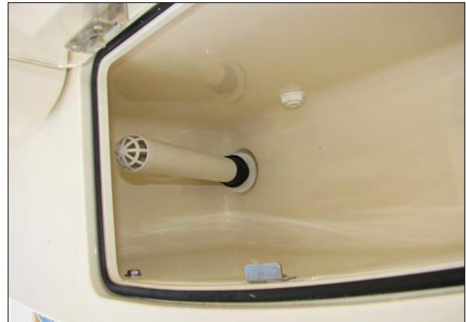
Typical Baitwell Standpipe & Drain Fitting
