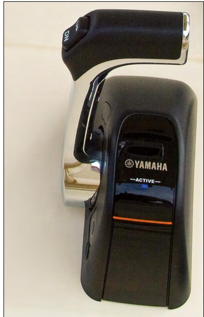
Yamaha Single Engine Binnacle Style Electronic Control
