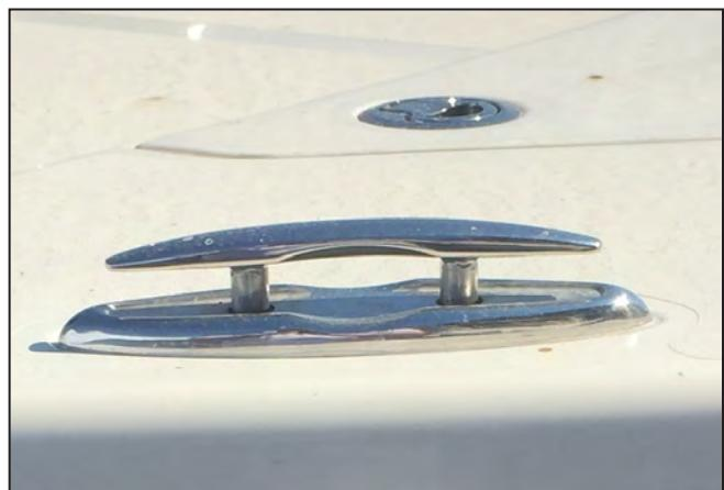
Typical Retractable Cleat In Mooring Position
