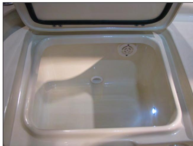
Typical Baitwell Drain, Overflow & Light
