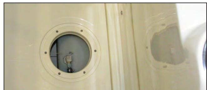
Typical Fuel Withdrawal Tube & Anti-Siphon Valve
