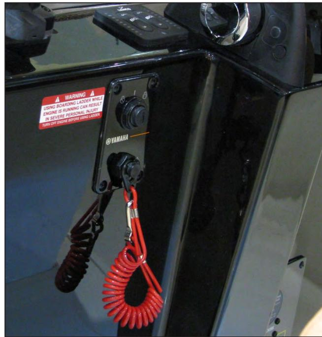
Typical Engine Stop Switch & Lanyard
