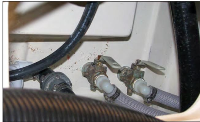
Typical Raw Water System Thru-Hull Valves
