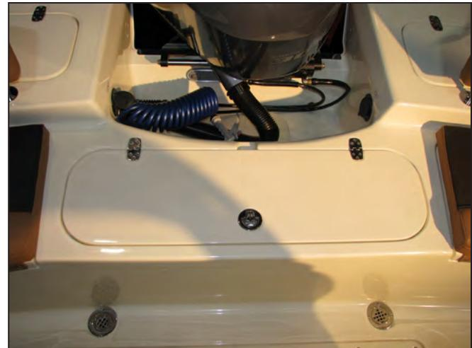
Typical Stern Release Well Hatch & Cockpit Scuppers
