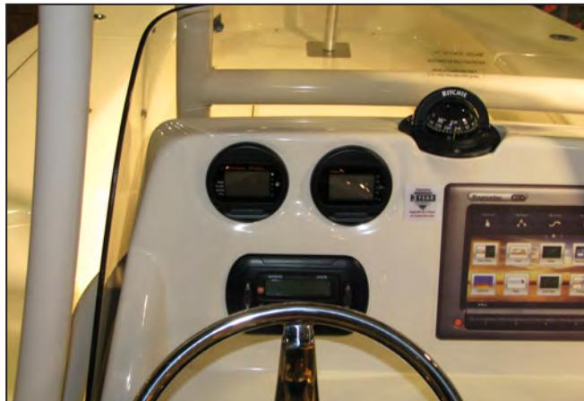
Typical Outboard Engine Instrumentation
